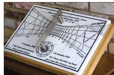
Polar sundial with analemma curves in order to provide civil time. Created by Dan O'Neal for the city of Santa Avelina in Guatemala.
