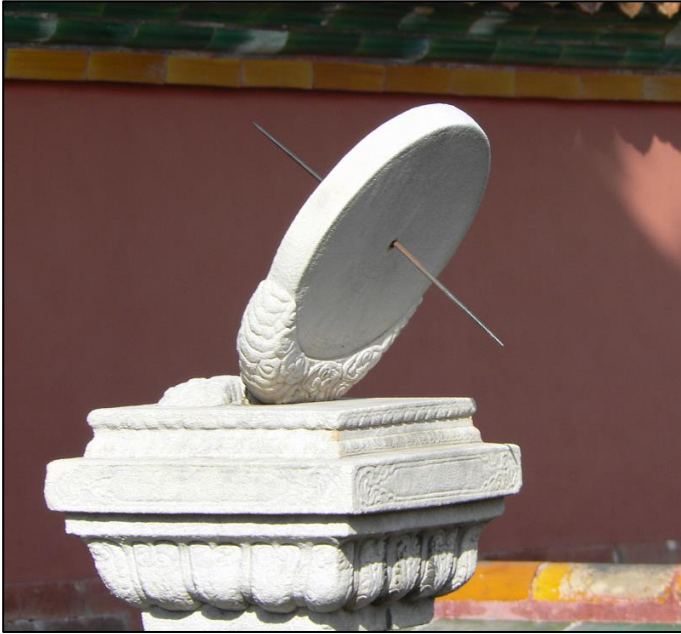
Left: one of the three equatorial sundials made in white marble, visible at the Forbidden City, Beijing, China.
