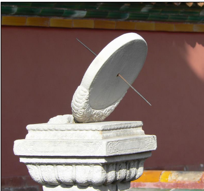
Left: one of the three equatorial sundials made in white marble, visible at the Forbidden City, Beijing, China. A single style emerges on both sides to allow reading time all year long.
